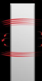
ICON contains DUAL-THERM technology that is two different heating systems in a single product: convection makes it possible to quickly reach the required comfort level in the room while radiant heating ensures that the front surface transmits constant and even comfort.
